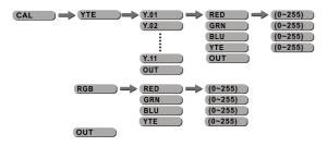
Press **[ENTER]** button to enter the password confirmation, to enter the correct password < UP + DOWN + UP + DOWN > Key, press the **[ENTER]** in, the correct password will enter show submenu
